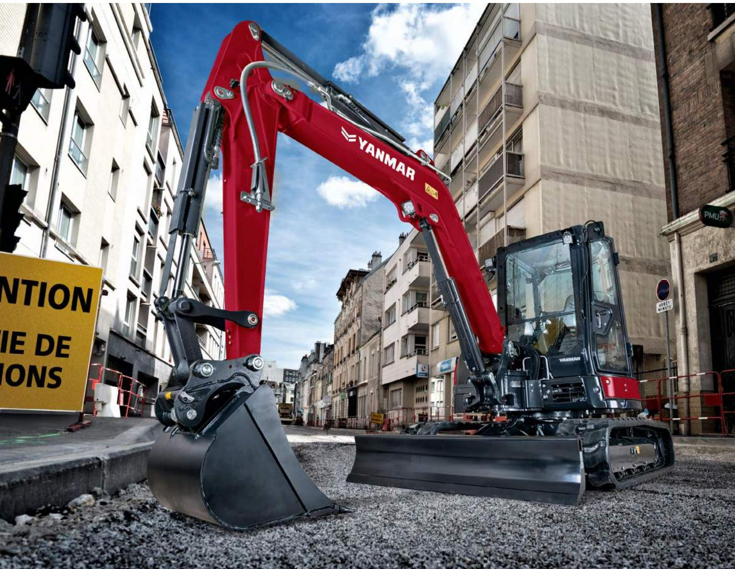
The Vi057-6B benefits from an improved powerline: the combination of the new more powerful engine new Stage V powerful engine with Diesel Particulate Filter, the hydraulic pumps (+ 14 %) and a new control valve improve the cycle-times by more than 10 %.
