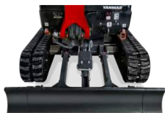
Extended undercarriage: 1170 mm
