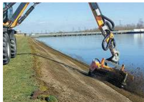
bema 25 with bema Weed brush (special attachment)
