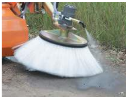
Rotary side brush with a water spray unit
