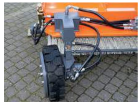
More efficient - steerable wheel-drive (hydraulic)
