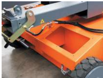
Machine casing with integrated water tank
