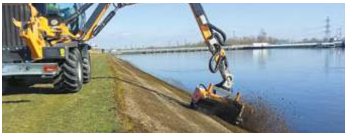
Sweeper built from the modular kit: bema 25 with bema Weed brush, without collection container, excavator mounting (special construction)
