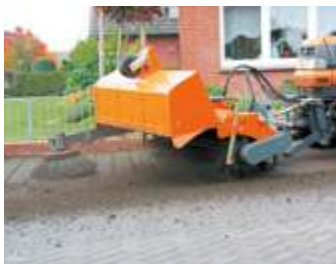
bema Sweeper equipped with bema Weed brush and rotary side brush
