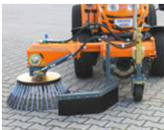
Flexible thanks to telescopic lateral movement (300 mm)
