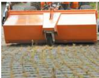
Weeds are directly picked up into the collection container
